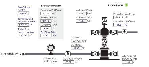
Real-time tile shows current values, status, and results in preferred unit of measure. A technician with authorization can tune the controller function that controls injection gas rate and pressure.
