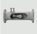
NUFLO cone meters feature inherent flow conditioning that eliminates straight-run pipe resulting in a weight-saving compact installation. The fabricated design enables diverse pressure ratings, sizes, and alloys of choice.
