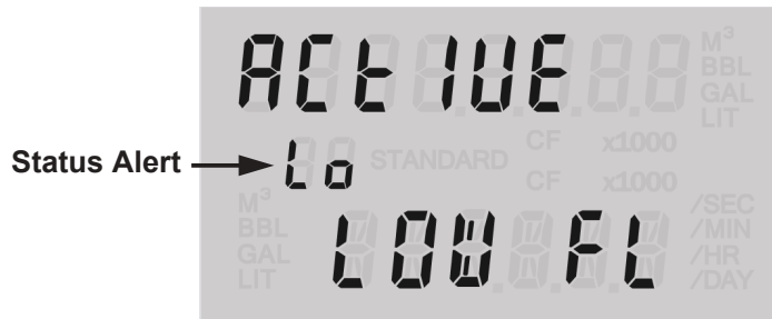
Figure 1.7—Turbine flow alarm display
