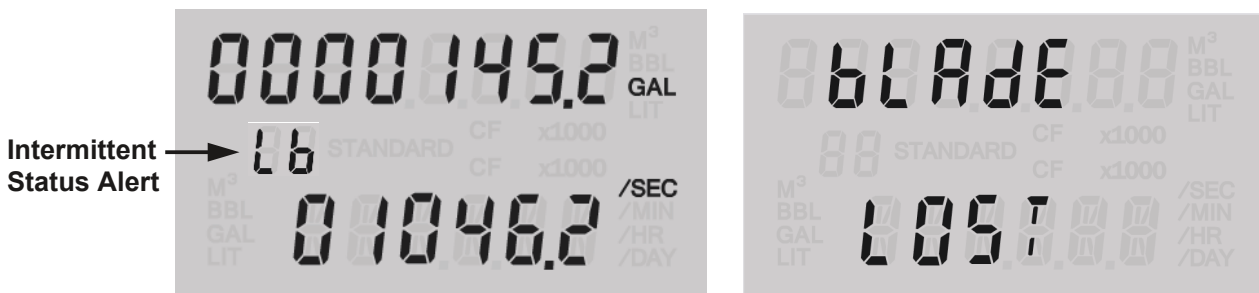
Figure 1.8—A turbine health alarm message (right) is preceded by a momentary two-digit status alert upon detection of a meter health vulnerability such as a missing or lost blade.
