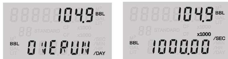
Figure 1.4—A flow rate overrun can be alleviated by using the X1000 unit selection for displaying rate.
