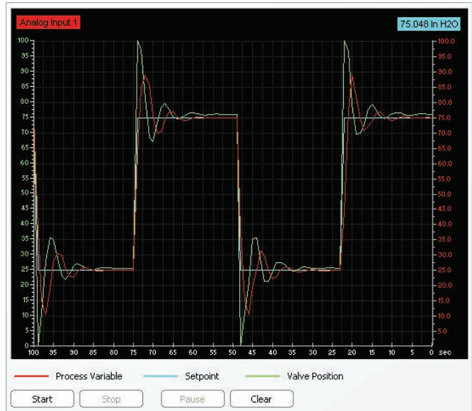
PID controller tuning tool in the QRATE Scanner 3000 series flow computer.
