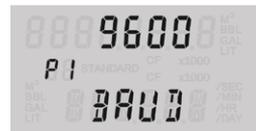
6. Use INC to advance to the desired baud rate. Tap ENTER to save the selection and exit the menu.
