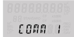
2. Use INC to advance to Comm 1. Tap ENTER to enter the menu. A cursor will flash in the top row of the LCD. "P1" indicates port 1 is being configured.
