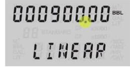
6. Tap STEP to advance the cursor to the numeric entry. Use INC to select the value of the flashing digit.
