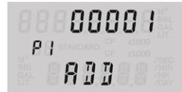
4. If the slave address contains more than one digit, use STEP to advance the cursor to the left and use INC to change the value.
