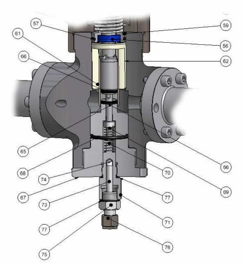
The Bottom Plug Assembly is unscrewed from the Cell Sampler Body using the 'C' Spanner provided in the Special Tool Kit. Note the location of any shims located between the Bottom Plug and the Cell Sampler Body. These will be retained on the Bottom Plug by 'O' Ring (68).
