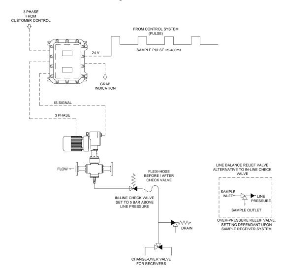
The Check Valve will normally be set to 5 Bar above the maximum line pressure, ensuring that this is sufficient to allow for any additional pressure increase created by thermal expansion when any isolating valves are closed and the effects of trace heating and or solar energy. If the cracking pressure is set too low, the valve may open under adverse conditions, causing the Sample Receiver System to overfill and the sample to leak through the relief valve to atmosphere.
