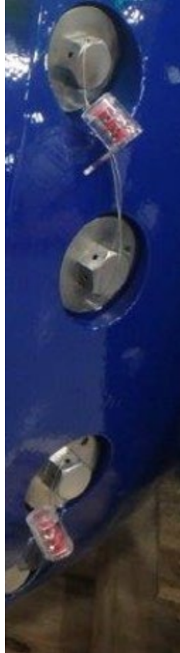
Figure 8.5—Seal wire on meter body
