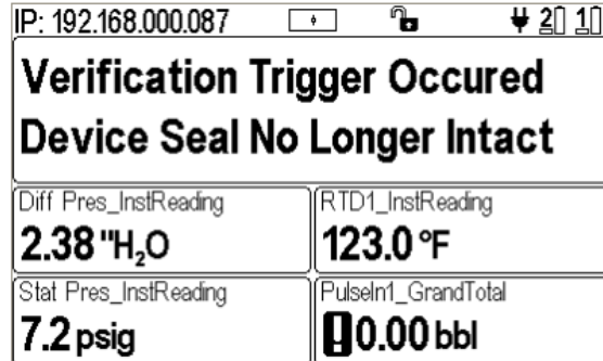
Figure D.9—Software Seal broken due to VTE (Verification Triggering Event)
