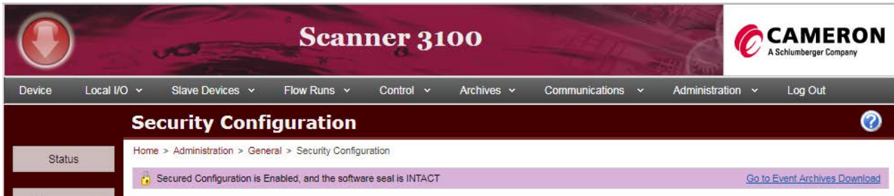
Figure D.10—Software Seal intact on Web Interface
