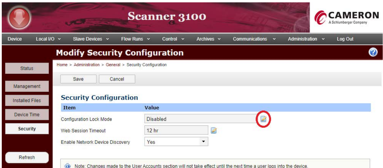
Figure 1.12—QRATE Scanner 3100 Web Interface Security menu
