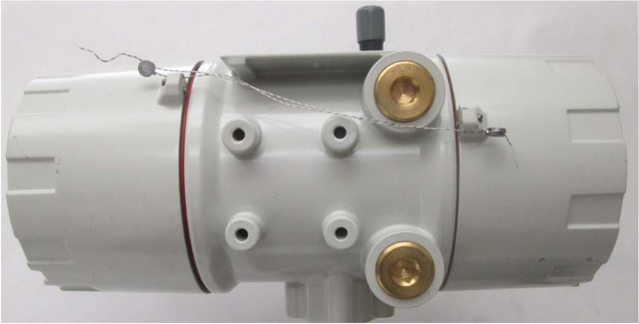
Figure D.7—Seal applied to QRATE Scanner 3100 without requirement for removable batteries
