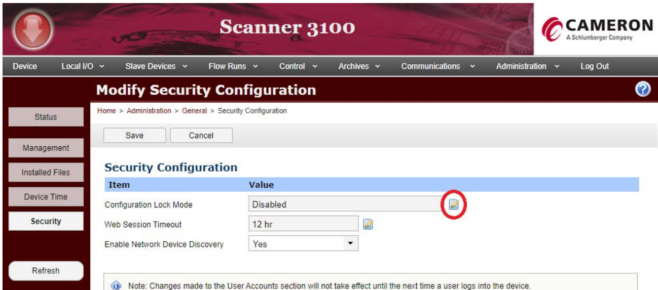
Figure D.5—QRATE Scanner 3100 Web Interface Security menu
