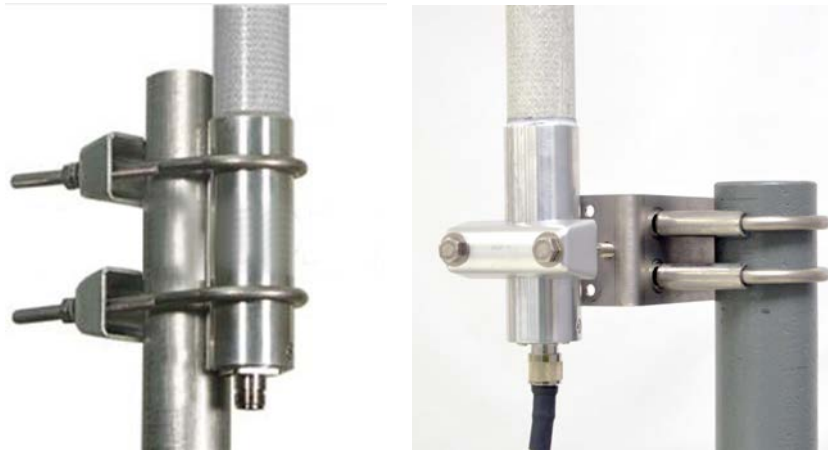
Figure 4.3—(Left) Standard antenna mounting bracket for outside pipe diameters up to 2-in. and (right) alternate antenna mounting bracket for outside pipe diameters of 2.375-in.
