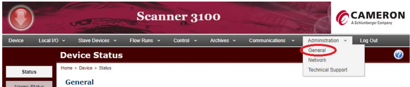
Figure D.3—QRATE Scanner 3100 Web Interface directions to Device Status screen
