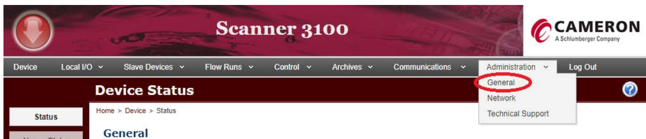
Figure 1.10—QRATE Scanner 3100 Web Interface directions to Device Status screen
