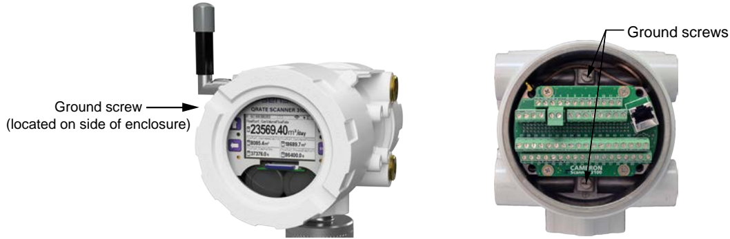
Figure 3.2—External and internal ground screw locations
