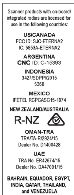
Figure 2.7—Radio frequency compliance label applied to the Scanner 2100 enclosure (content may change without notice)
