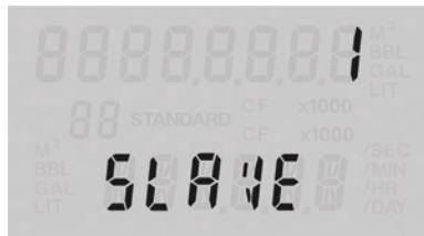
Figure 4.6—In configuration mode, the parameter to be configured is displayed at the bottom of the LCD and the setting for that parameter is displayed in the top LCD.
