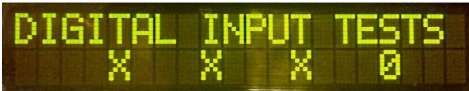
Figure 24 - The Digital Input test screen from the IO test menu. Note: In this example only, the last digital is an input. The rest have been configured as either outputs or as a grab signal.
