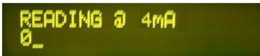
Figure 28 - Set 4mA calibration point during DAC calibration routine.
