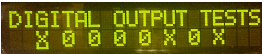
Figure 25 - The Digital Output test screen from the IO test menu. Note: In this example only digitals 2, 3 4, 5 and 7 are outputs. The rest have been configured as either inputs or as a grab signal.
