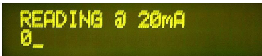
Figure 29 - Set 20mA calibration point during DAC calibration routine.
