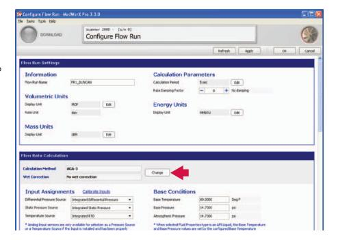
5. From the Change Flow Run Calculation Methods screen, select the Fluid Properties Calculation Method that is appropriate for the type of fluid being measured.
