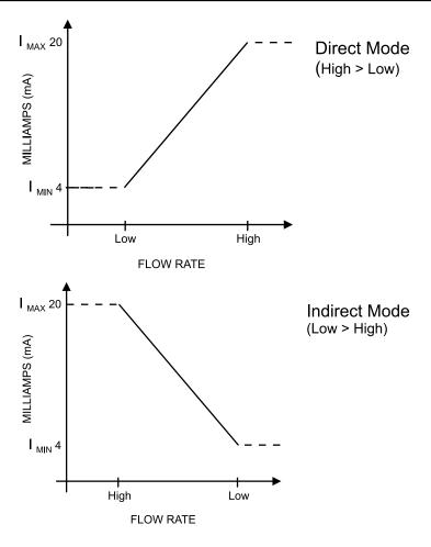
Figure 4.28—Two options for configuring a 4-20 mA output
