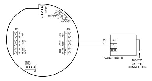
Figure 2.12—RS-485 output (connection to laptop with 25-pin converter)
