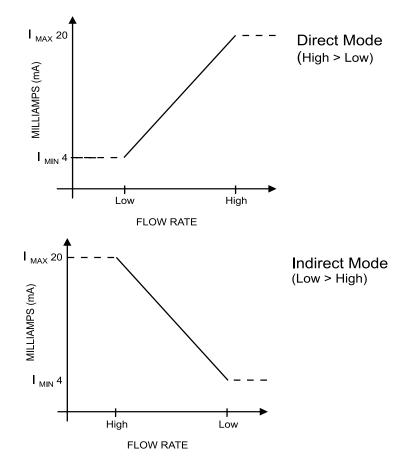
Figure 3.1—Two options for configuring a 4-20 mA output
