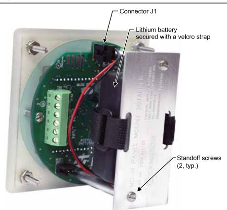
Figure 6.1—Lithium battery replacement
