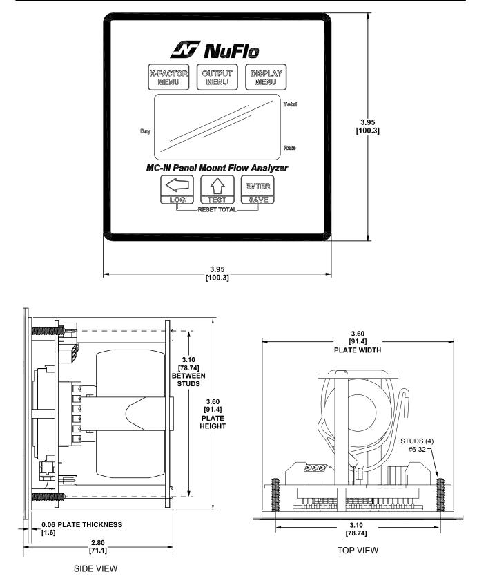
Figure 2.1—Typical mount dimensions in inches (millimeters)
