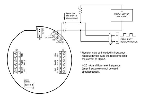
Figure 2.9—Flow meter frequency (amp & square) output wiring
