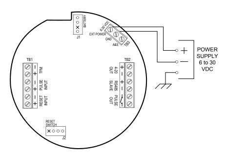
Figure 2.2—External power supply wiring
