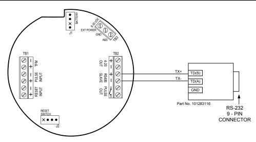
Figure 2.11—RS-485 output (connection to laptop with 9-pin converter)
