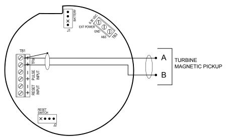
Figure 2.3—Flow meter input wiring
