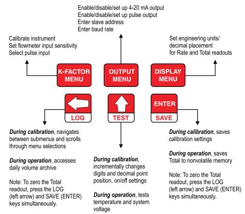
Figure 1.3—MC-III Panel Mount keypad functions
