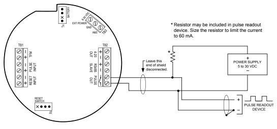
Figure 2.7—Pulse output wiring
