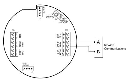
Figure 2.10—RS-485 output (permanent connection)
