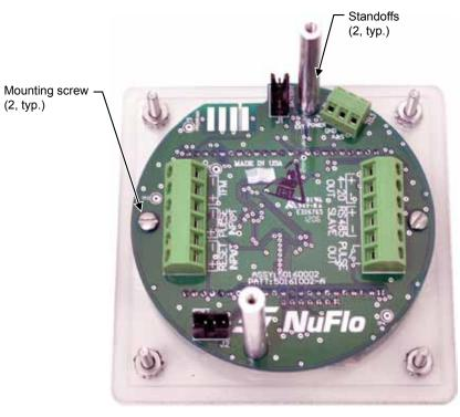
Figure 6.2—Removal of circuit assembly
