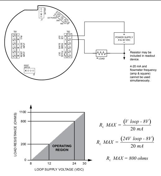
Figure 2.8—4-20 mA rate output wiring
