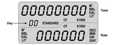
Figure 1.2—LCD display showing location of the Total, Rate, and daily index (Day) displays. Only the units of measurement selected for displaying total and rate will be visible during normal operation.
