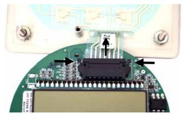
Figure 6.4—To release the ribbon cable from the connector, press in on the side tabs of the connector and gently pull forward (top arrow).
