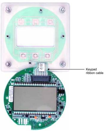
Figure 6.3—Keypad ribbon cable connection
