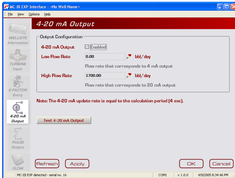
Figure 4.28—4-20 mA Output screen
