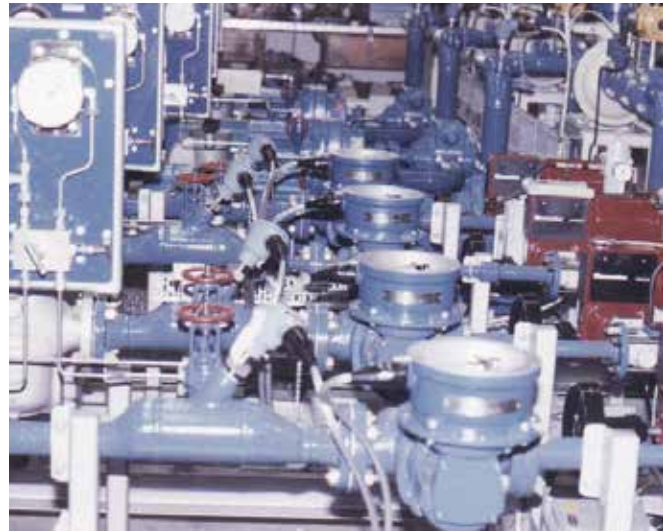
JISKOOT in-line blending system for lube oil
