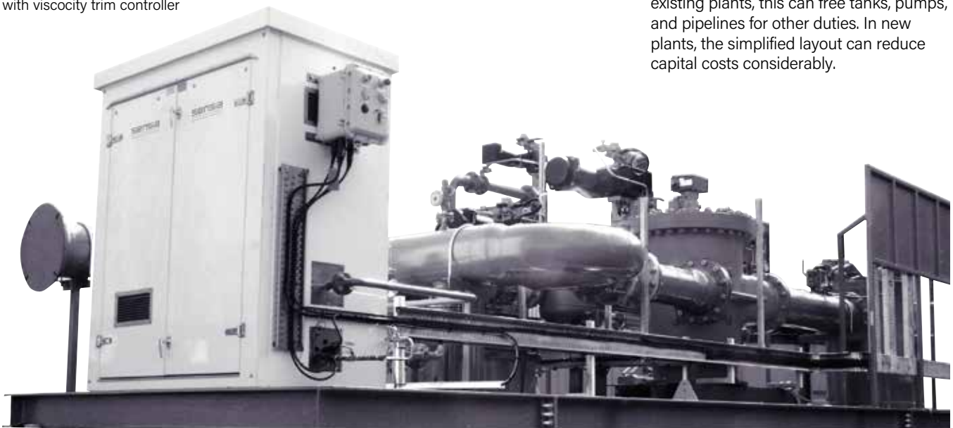
JISKOOT in-line blending system with viscosity trim controller
