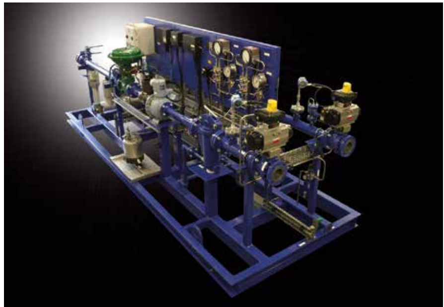
JISKOOT in-line blending system for fuel oil
