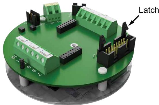
Figure 5.5 - Latch securing the ribbon cable
