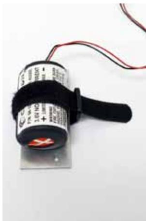
3. Insert the battery, then pull the loose end of the strap over the battery and through the buckle.
