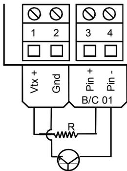
Resistance is calculated based on the voltage ( $V_{tx}$ , 10V or 24 V) and the threshold.
