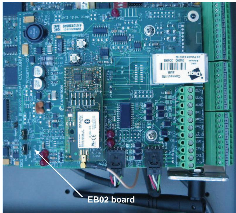
Scanner 1131 with EB02 Ethernet-Bluetooth board installed
