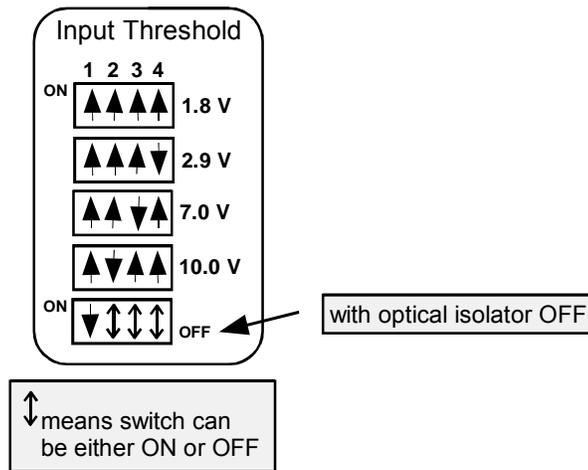
The “OFF” threshold selection is used when the channel is being used in non-isolated mode, as a digital output channel, or when the channel is not being used at all. Turning it off will conserve the 2 mA per channel required to power the optic isolator.
