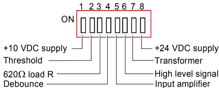
The following diagram illustrates the **ON** and **OFF** positions as they are used in the pulse input diagrams:
