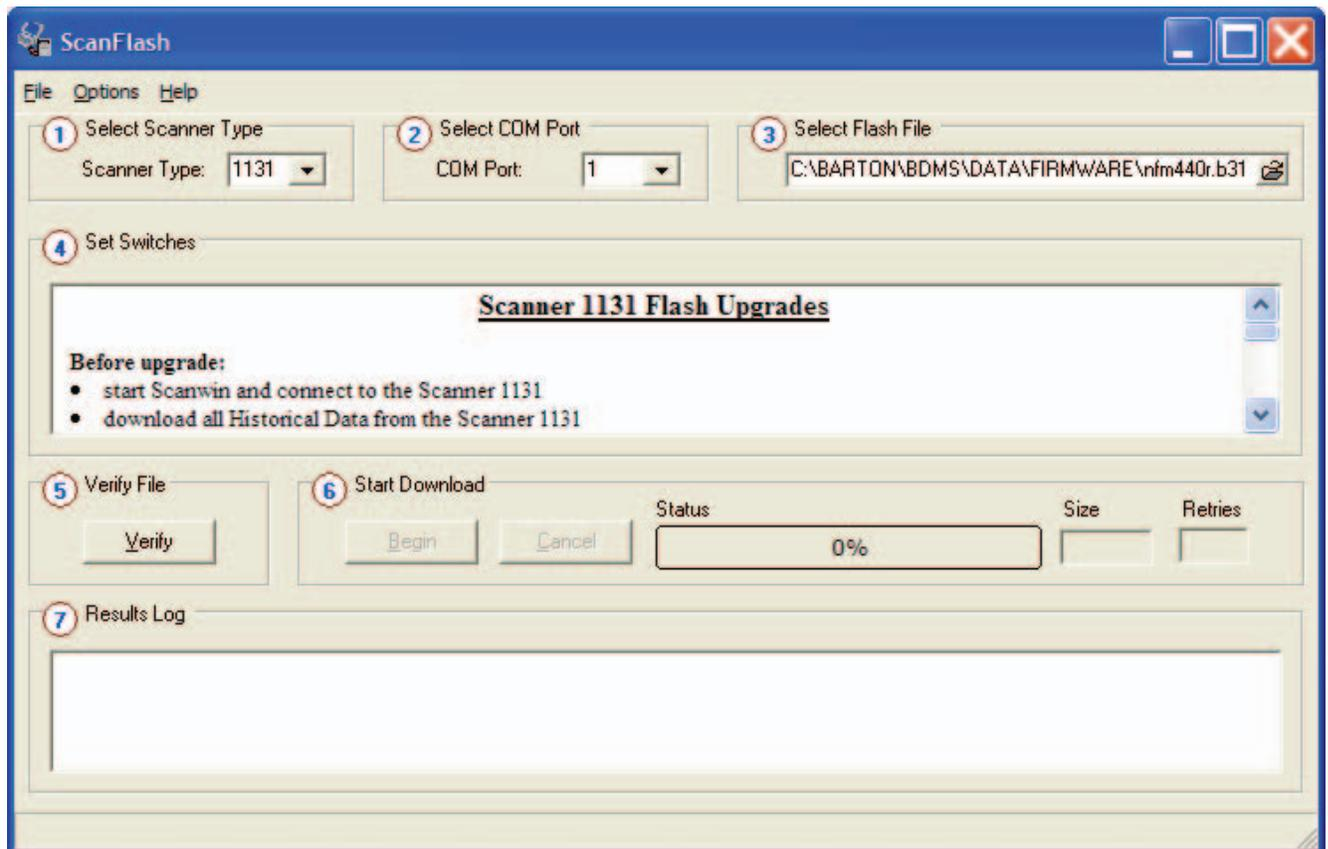
ScanFlash step 4 is Set Switches – The dialog box items 1 thru 4 describe the order for the power and program erase PE switches.
