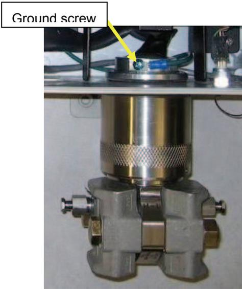
Proper positioning of the DPE+ transducer
