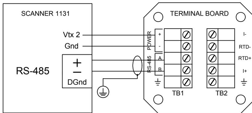
Up to two MVX-II instruments can be powered from the Vtx2 (12 Vdc) terminals of the Scanner 1131. RS-485 +/- terminals for A02 are #1 and #2. RS-485 +/- terminals for A04 are #14 and #15.
