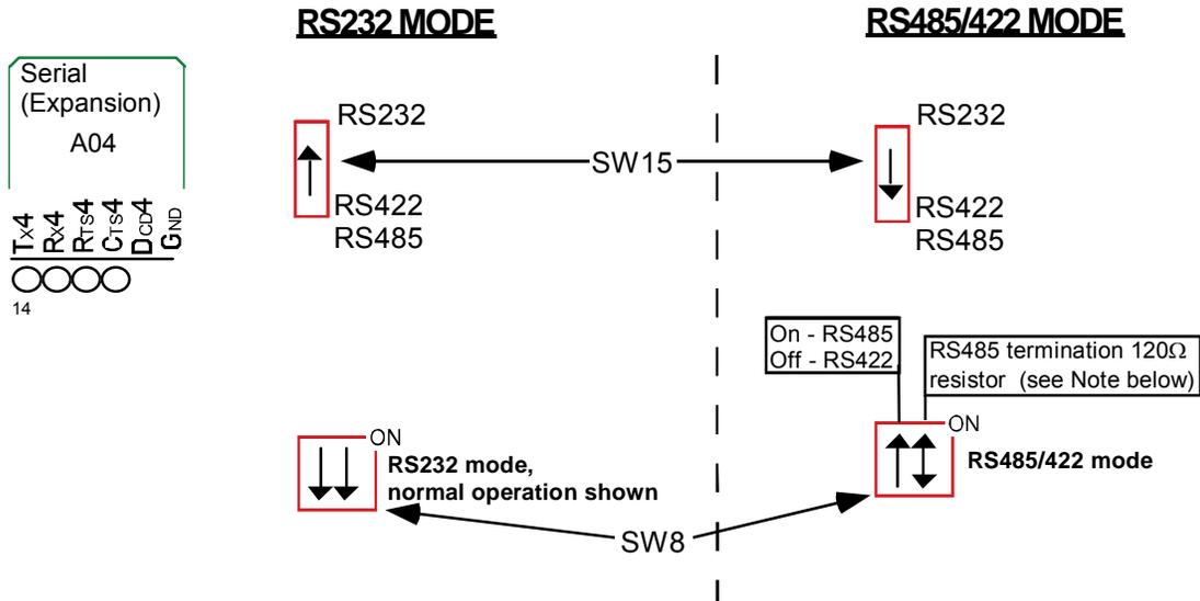
**Note:** \* If the Scanner is LAST in the 485 loop, the 120Ω termination switch should be left in the "**ON**" position; place switch in the "**OFF**" position if it is not.
