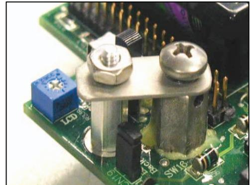
When it is required to be LOCKED, the screw must be tightened until a **CLICK** is heard. Continue tightening the screw until it is possible to insert the sealing wire through the hex bar stock/screw. Sealed, it looks like the following:
