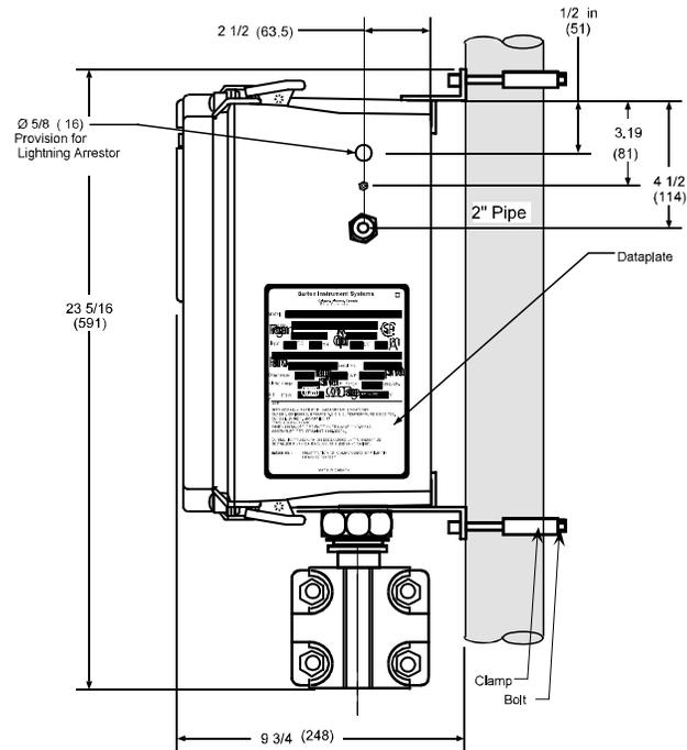
2. DPE mounting standard 2-1/8" spacing 1/4" NPT process connections.
