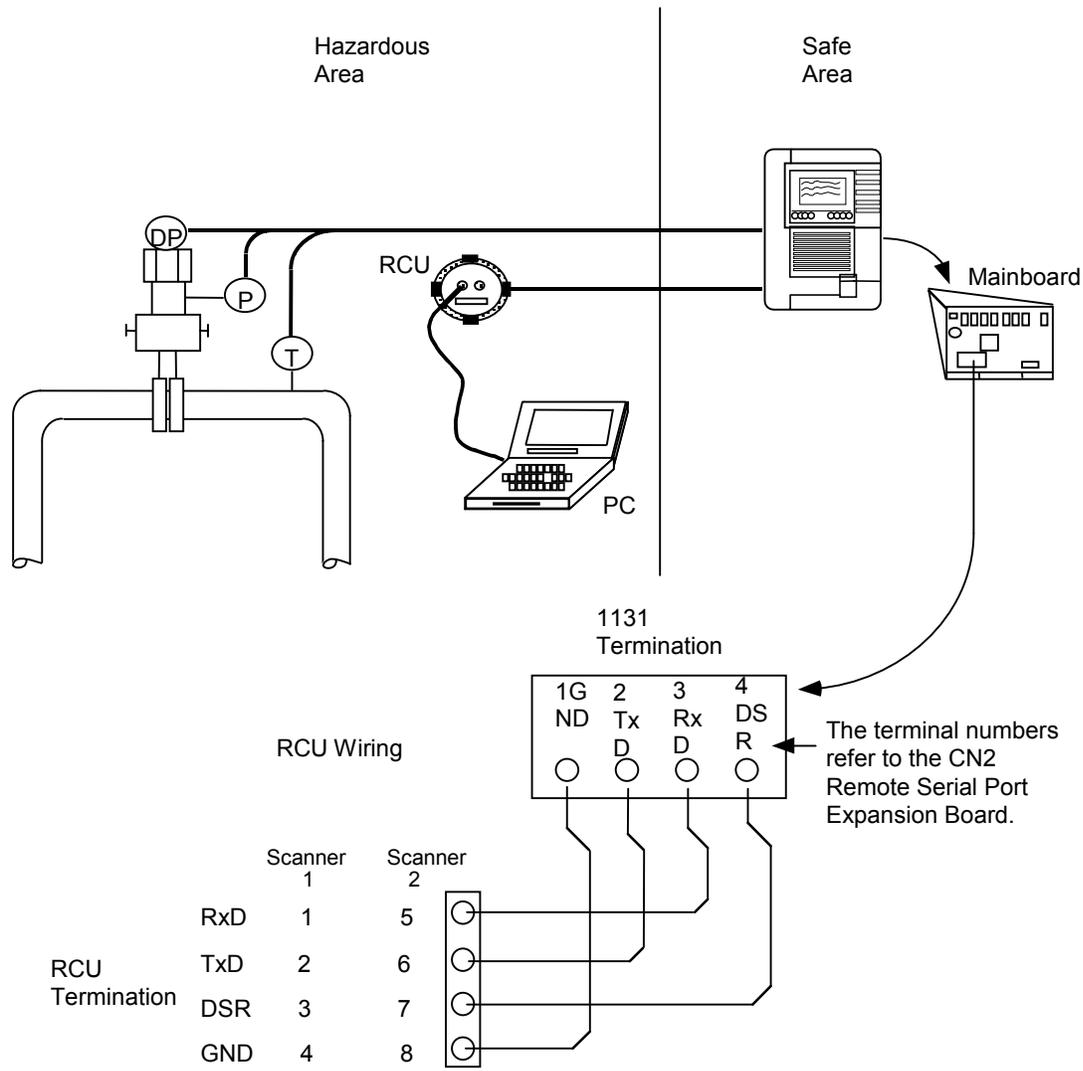
**Note:** The user may also use the CN3 Communications Accessory Board or the second serial port of the main board if the port is assigned to a remote console.
