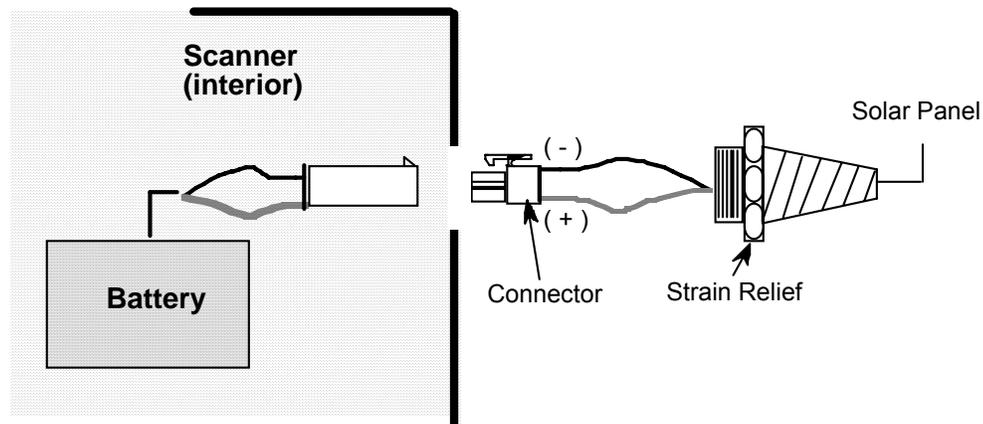
The battery input (charging) cable has a weatherproof strain relief and a quick-release connector that connects the battery to the solar panel's cable.
