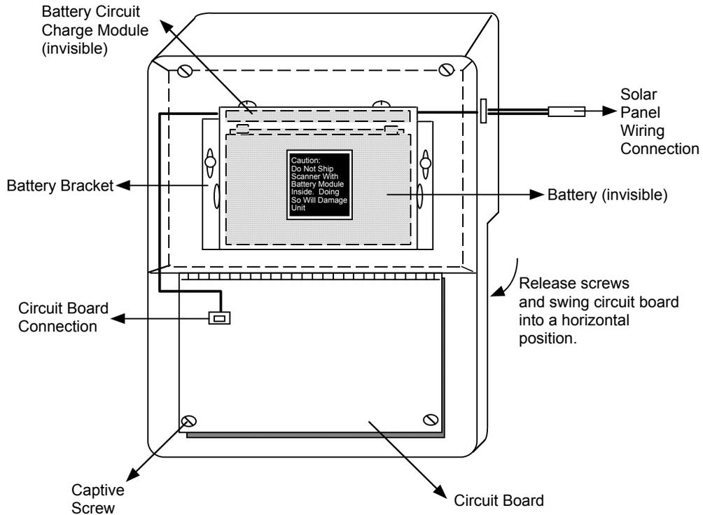
The battery output cable is plugged into a connection on the back of the main circuit board.
