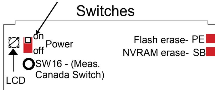
To turn the unit on, place the Power Switch in the **ON** (up) position. This causes a **Power on restart**. The Power on restart interrupts the flow calculations, but does not affect the configuration or historical data. The display will show:
