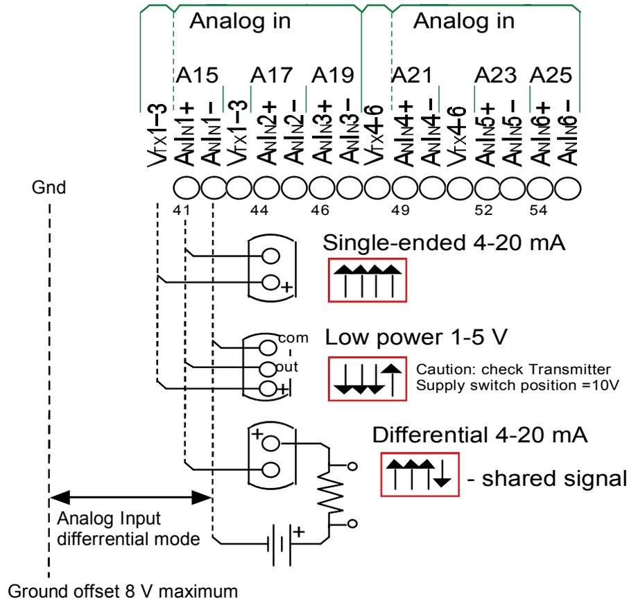
**Note:** The **TOTAL** +10 V transmitter output (e.g. Vtx10, Vtx1-3 **and** Vtx4-6) is 15 mA.
