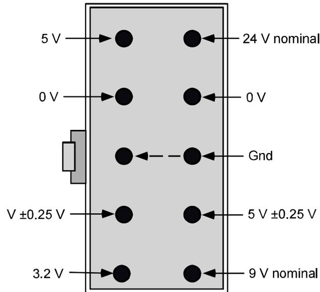
The battery should be charged with a 15-28 Vdc supply at 750 mA maximum. The battery should be charged during storage and before installing in the flow computer. Voltage should be over 13 Vdc half an hour (30 minutes) after the power is removed. Replace battery if voltages are low to zero. Recharge questionable battery and recheck the connector voltages.
