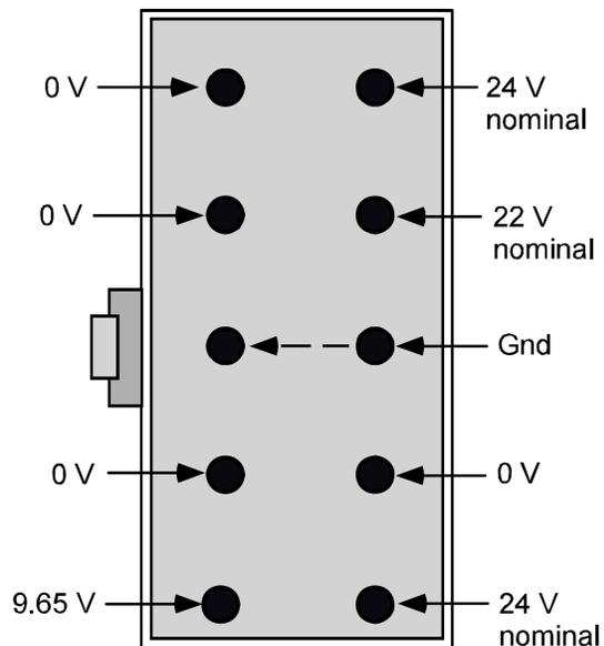
The following diagram shows the approximate readings obtained when the power supply is plugged into the main board:
