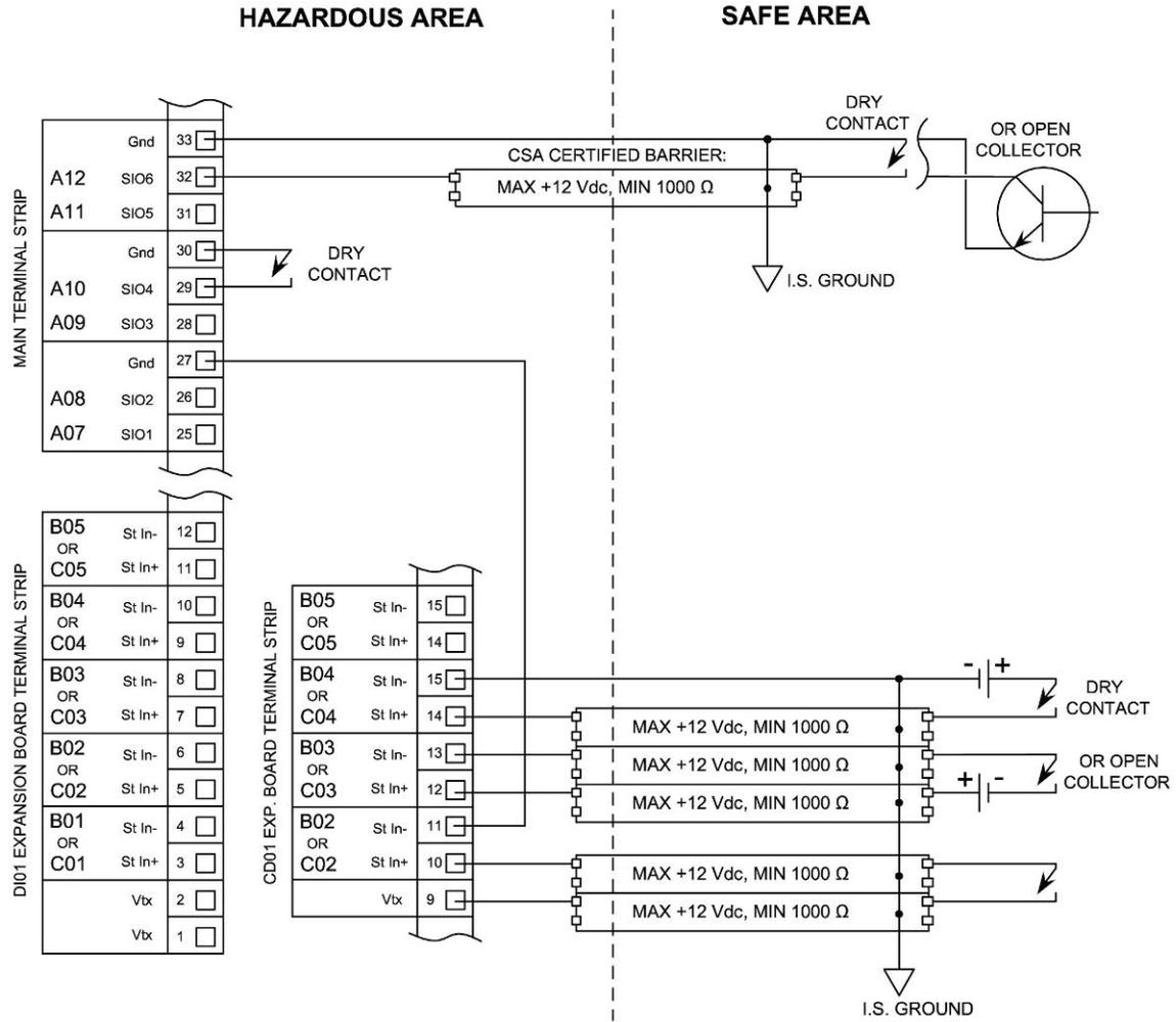
STATUS INPUT WIRING AS SHOWN CAN BE CONNECTED TO ANY OR ALL DIGITAL INPUT / OUTPUT RESOURCES SHOWN.
