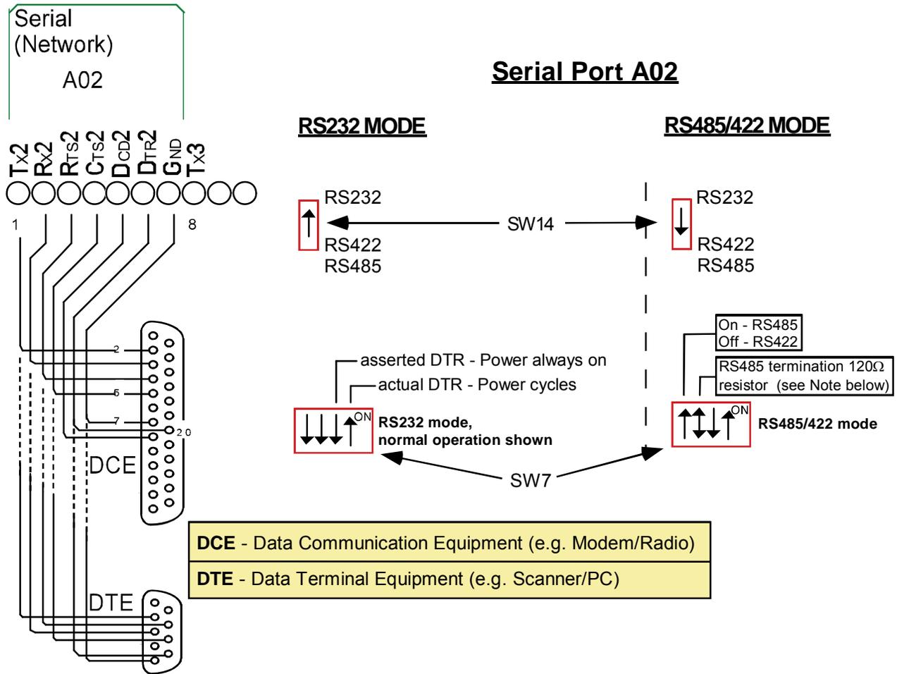
**Note:** \* If the Scanner is LAST in the 485 loop, the 120Ω termination switch should be left in the "ON" position; place switch in the "OFF" position if it is not.
