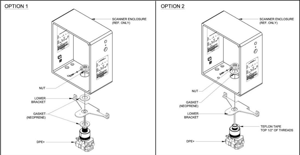
Install a gasket between the enclosure and the bottom bracket, and another gasket between the bottom bracket and the DPE+ adapter.
