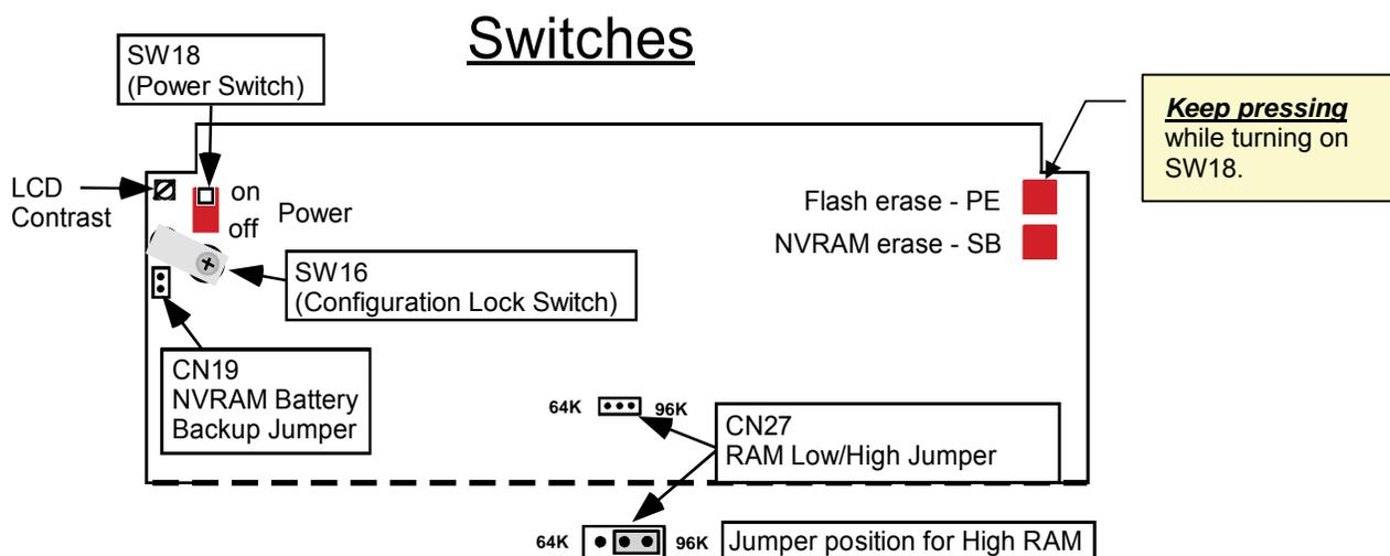
The **Flash Erase** switch, labeled “**PE**” for **Program Erase**, is located at the top right hand corner of the main board. It is used by the system to initiate the process of re-installing its own firmware. The function is
