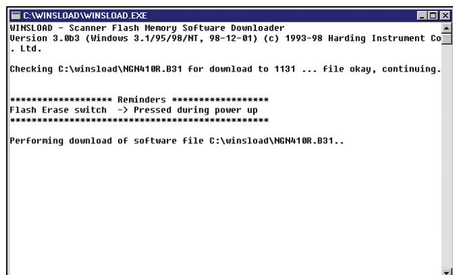
WinsLoad begins to erase the ROM. When that is done, it then begins to upload the new firmware to the Scanner while displaying the percentage of the file that has been transferred.
