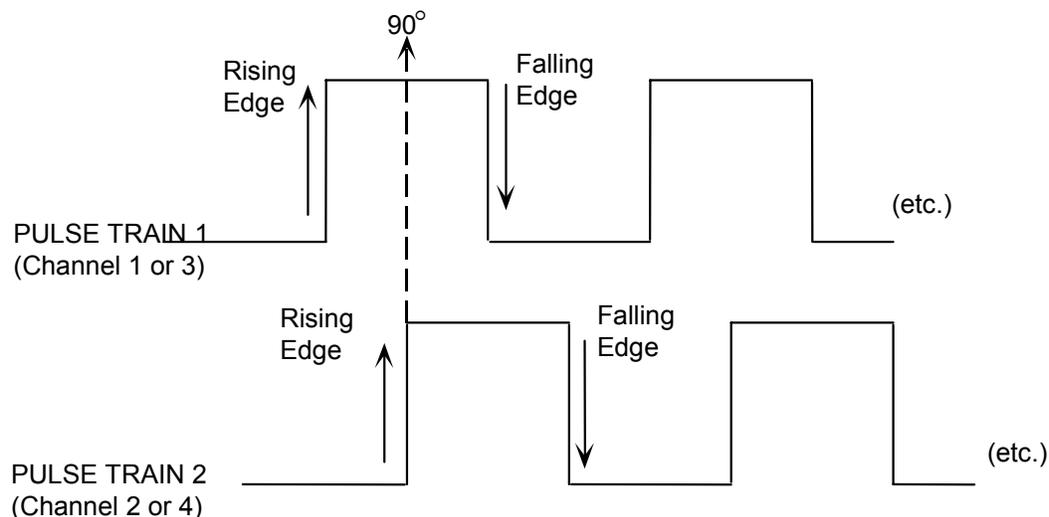
The fact that Pulse Train 1 is leading Pulse Train 2 is interpreted by the Scanner as flow in the FORWARD direction. If Pulse Train 2 were leading Pulse Train 1, it would be REVERSE flow.
