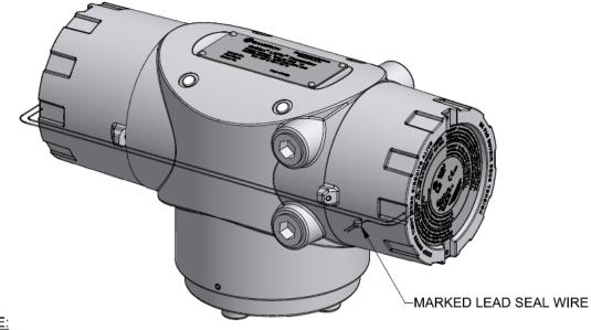
NOTE: THE LEAD SEAL SHALL HAVE EITHER A MARK DEFINED BY THE USER OR A MARK OF A NOTIFIED BODY.
