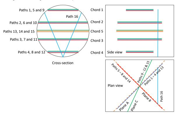
Figure 5.1—Illustration of chord, plane, and path
