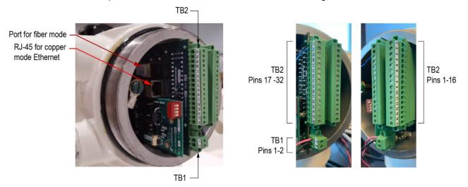
Figure 3.2—User terminations, rear view
