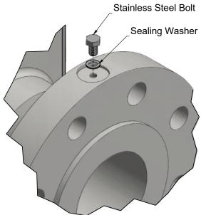
Figure 2.1—Stainless steel bolt and washer in tapped hole of meter body end flange
