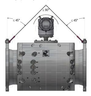
Figure 2.2—Proper sling attachment
