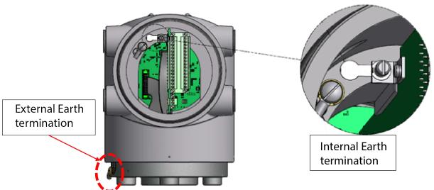
Figure 3.9—Earth points on transmitter body (refer to Table 3.7 for isolated ground connections to be made by user)
