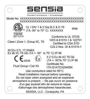
Figure 1.2— Meter body approvals nameplate example
