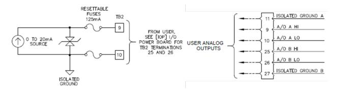
Figure 3.7—Typical analog output
