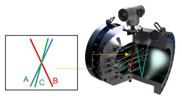
Figure 4.2—Three paths per chordal plane as used in the Caldon SVM
