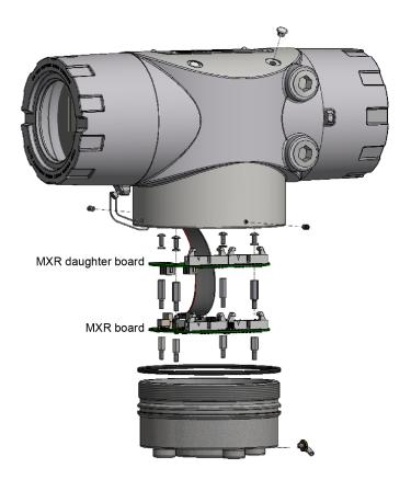
Figure 6.7—Disassembling the transmitter to access the MXR
