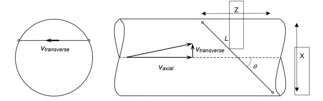
Figure 4.1—Illustration of the transit time principle
