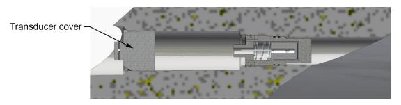
Figure 6.9—Transducer housing cross-section
