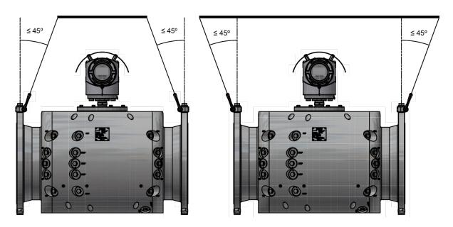
Figure 2.3—Hoist rings with a lifting bar above the electronics unit allow for uniform lifting.
