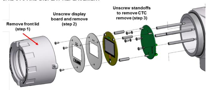
Figure 6.4—Disassembly views for CTC and display replacement
