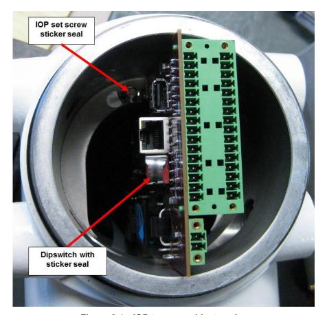
Figure 8.4—IOP tamper-evident seals
