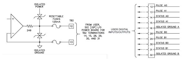
Figure 3.8—Typical digital signals
