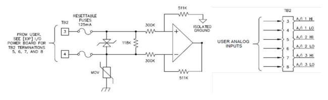
Figure 3.6— Typical analog input
