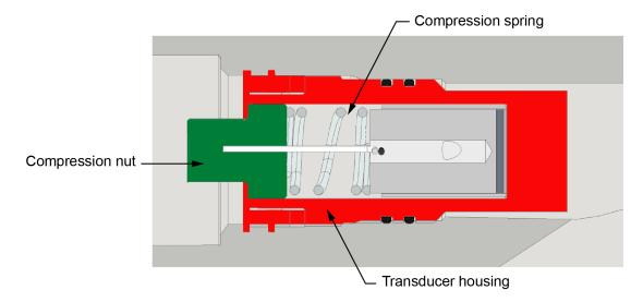
Figure 6.10—Transducer housing detail
