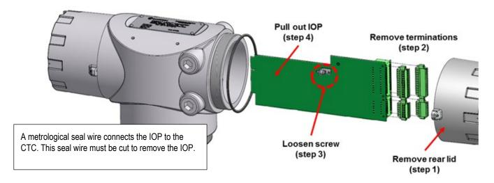
Figure 6.2— Disassembly views for IOP replacement
