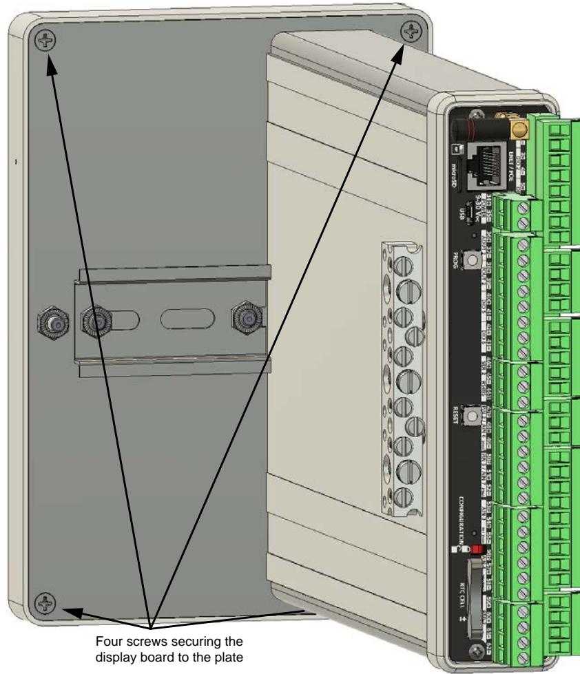
Figure 5.2 - Screws attaching the QRATE Scanner 3300 display assembly to the plate and main enclosure.
