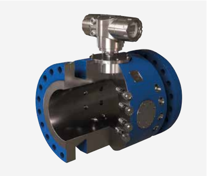
Eight-path chordal design that ensures accurate measurements without additional flow conditioners, even in flows containing swirl and asymmetry.
