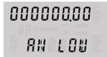
14. Tap STEP to select the right-most digit of the low-flow limit. Use INC to change the value of the flashing digit.
