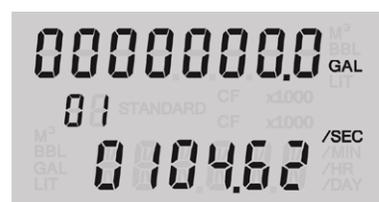
15. Tap STEP to switch to the numeric value entry. The rightmost digit will flash to identify the digit selected for change.
