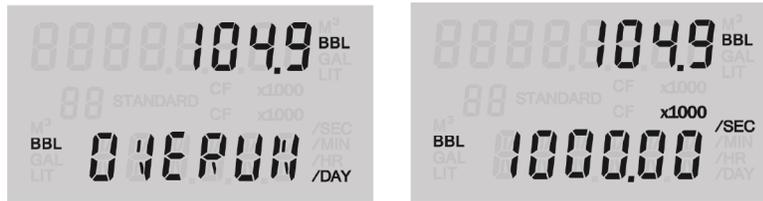
Figure 1.5—A flow rate overrun can be alleviated by using the X1000 unit selection for displaying rate.
