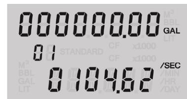
13. When all frequency digits are entered, tap STEP to move the flashing digit selector to the DECIMAL in the top row of the LCD (K-factor).
