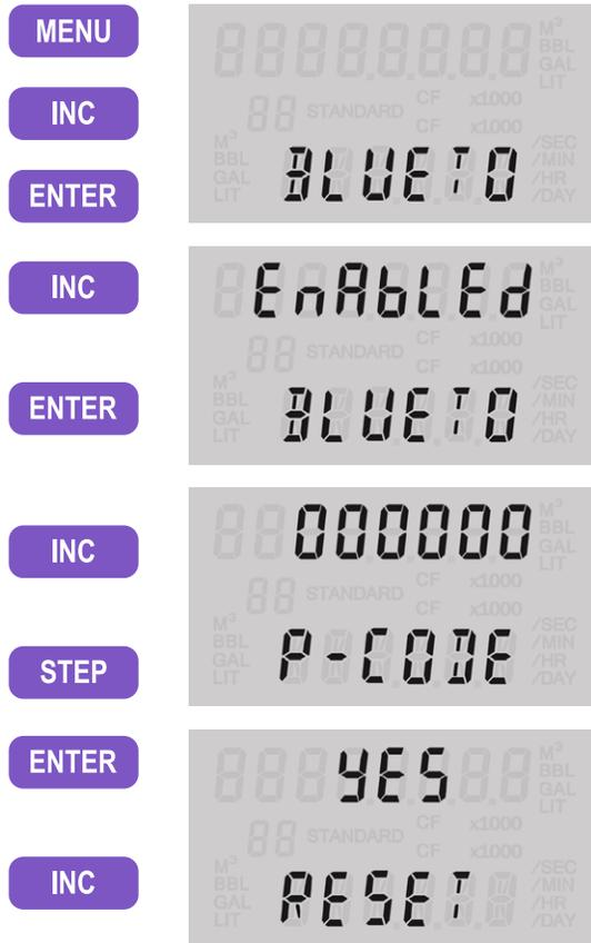
10. Tap ENTER to execute the selected action. **If resetting the module, wait until BT RESETTING disappears from the LCD and DONE appears on the top line. (CLEAR PHONE PAIRING will scroll across the bottom line of the LCD.)**
