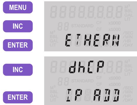
This Ethernet connection does not have a dedicated web interface. All settings are configured via the PC software for the MC Synergy. However, you can confirm the viability of the Ethernet connection by entering the IP address in a web browser.
