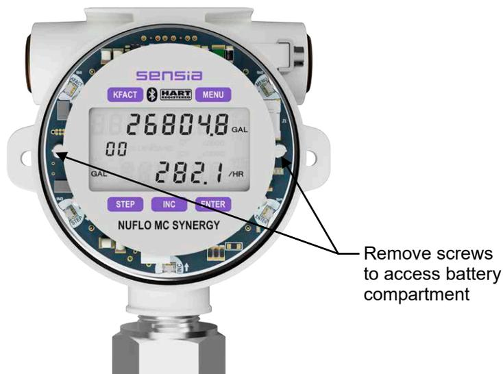
Figure 4.3—Removal of faceplate assembly
