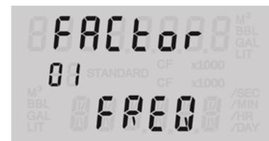
When the rightmost digit in the bottom row begins flashing, proceed to step 9 to enter the frequency value corresponding with calibration point 1.
