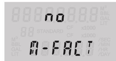
2. Tap ENTER to bypass the meter factor menu and continue on to the K-factor Type menu. Linear will display by default.
