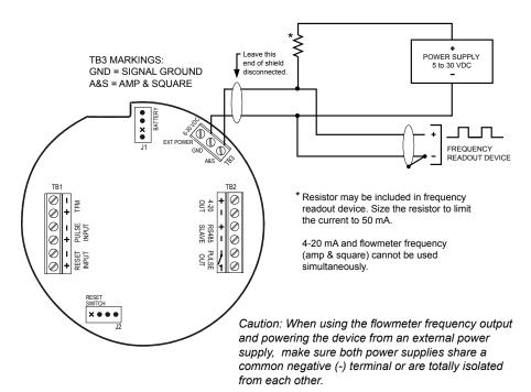
7. To configure the MC-III with software, connect the MC-III to a computer by wiring a converter cable to the RS-485 terminals of TB2. See page 12 for wiring diagrams.
