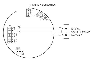
3. If an external power supply is to be used (the battery will provide backup power), wire the power supply to terminal block TB3.
