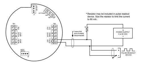
5. If a 4-20 mA rate output is to be used, wire the power supply to terminal block TB2. The power supply voltage required to power the current loop depends on the loop resistance. See an MC-III user manual for details.
