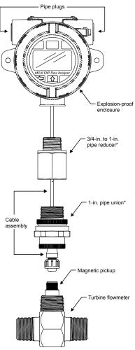
\* Pipe reducer and union are used in CSA-approved MC-III devices only.
