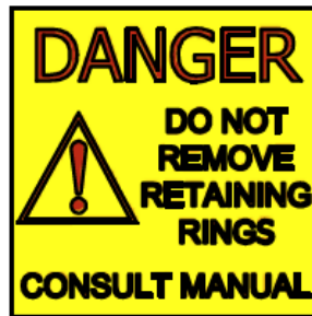
Figure 7-12 Retaining Ring Warning Sticker
