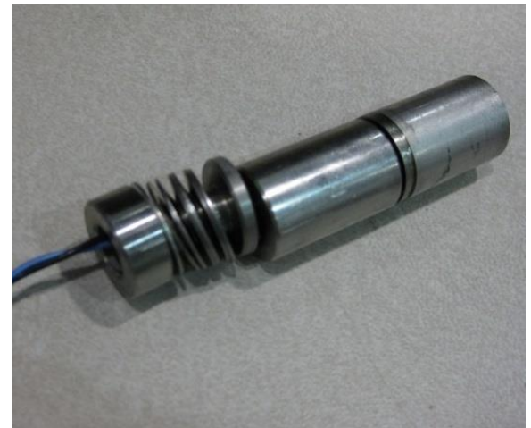
Figure 7-14 Transducer Internals (shown components are for 1.0 Inch housing – note that the spacer is next to the transducer)
