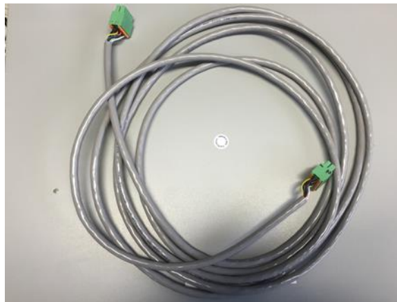
Figure 5-10: INSTRUCT Power Analyzer 5kV Voltage Sensor Signal Cable
