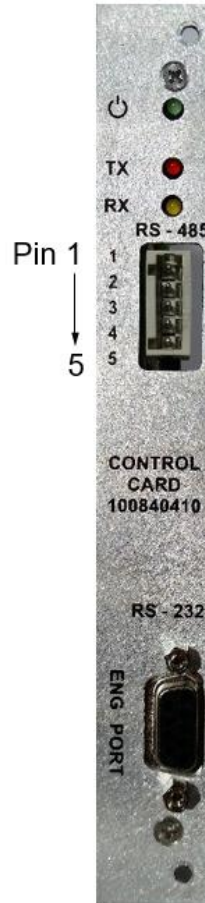
Figure 5-3: RS-485 Wiring Diagram
