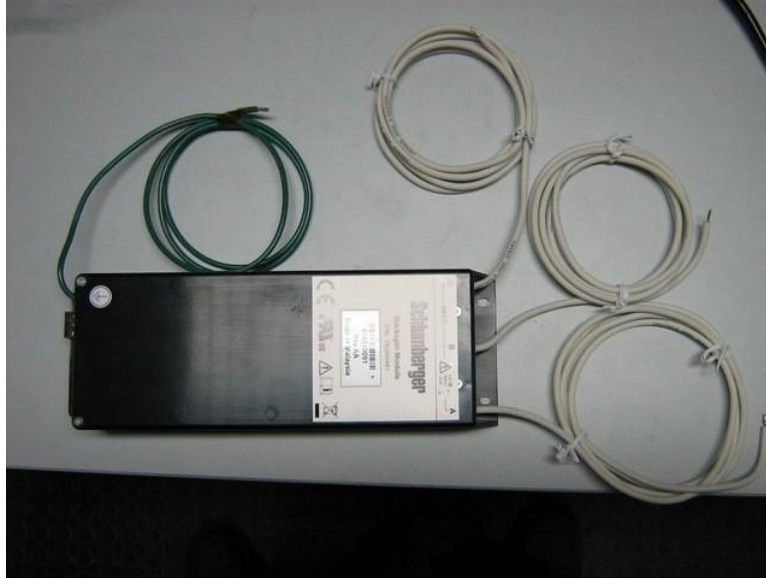
Figure 5-9: INSTRUCT Power Analyzer 5kV Voltage Sensor
